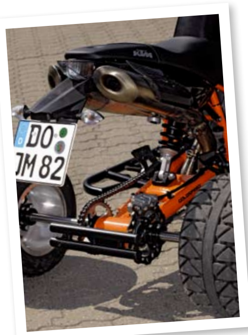
ABOVE: Check out the stainless rear axle and Brembo with wave rotor. E-ATVs (the "E" stands for company director Clemens Eicher) have been in development for 10 years and we've often seen them at France's famous 12 Hours of Pont de Vaux. But they've been on the market for only two years. BELOW: Welds and powdercoating are immaculate. Note the alternate lower shock mount.
